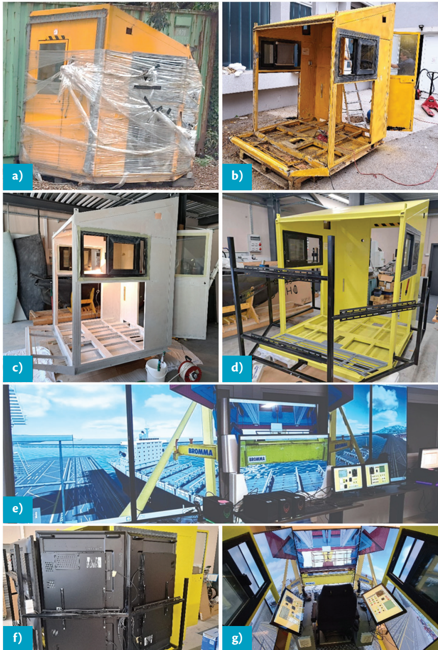
Figure 1. Crane Cabin Repairation and Modification Process: a) Dismantled crane cabin donated by the Port of Koper; b) Removal of glass surfaces and initial treatment of rusted metal; c) Protection and painting of metal components; d) Installation of supporting consoles for the large screen; e) Software setup and hardware calibration in the laboratory; f) Cabling and mounting of the large screen; g) Final appearance of the crane simulator.
